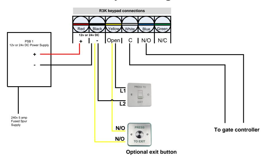
Access control system with magnetic lock & additional keypad
