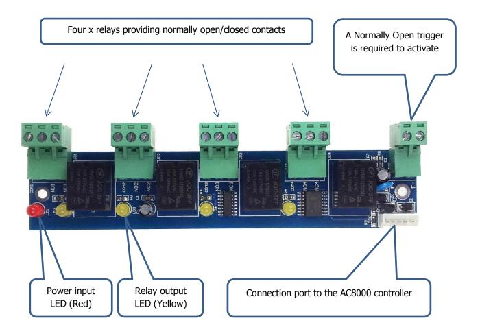
Example of the AC-FAB being activated by the alarm input, but also triggering one of the four relay outputs to activate a strobe light from 0-6000 seconds (1.66hrs)
