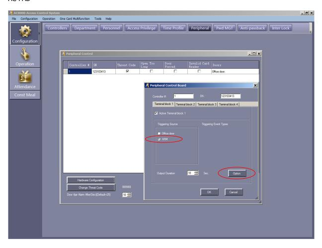
This configuration will trigger a Fire Alarm event via the software and also activate relay output number 1 indefinitely on the AC-FAB until the trigger is reset
