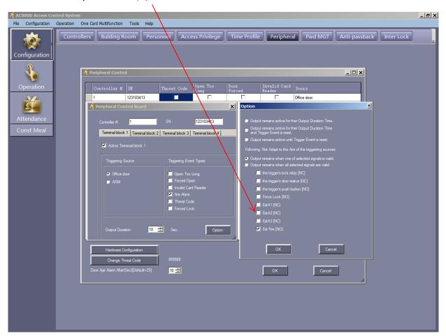
This configuration will trigger a Fire Alarm event via the software, the door status (Open or closed) as well as the exit button being pressed and activate relay output number 2 indefinitely on the AC-FAB until the trigger is reset
